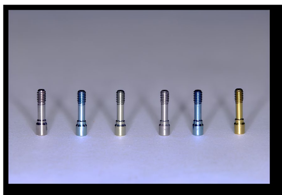
Fig. 2 Surface treatment of implant abutment screws. Left to right respectively, C, B, Y, A, AB, AY. C Control, B Blue, Y Yellow, A acid etched, AB Acid etched Blue, AY Acid Etched Yellow
