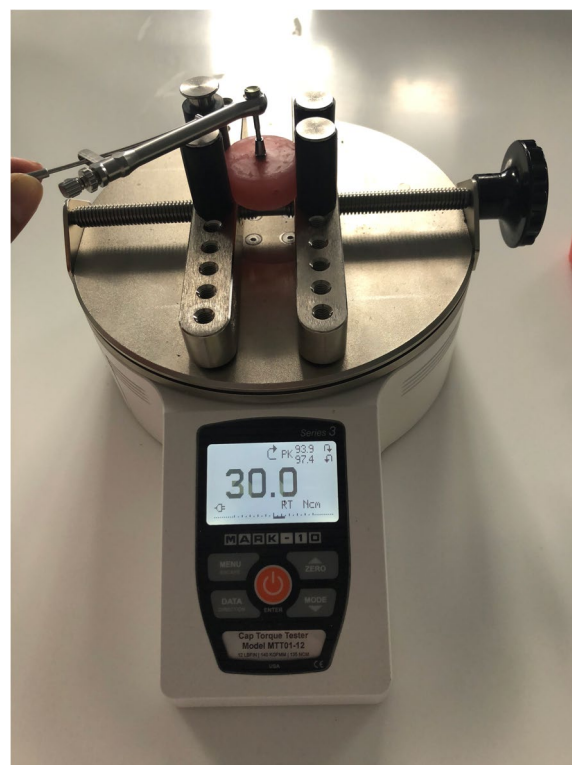
Fig. 3 Connection of implant-abutments and torque application
